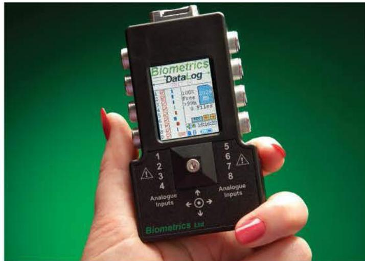
The **DataLOG MWX8** is the latest in data acquisition technology developed to meet the needs of researchers for portable data collection and ambulatory monitoring in human performance, medical research, industrial ergonomics, gait laboratories, sports science, and educational settings. The small, lightweight, battery operated unit incorporates a joystick, colour graphics LCD, Micro SD card interface, and a real-time wireless Bluetooth link to a PC.
