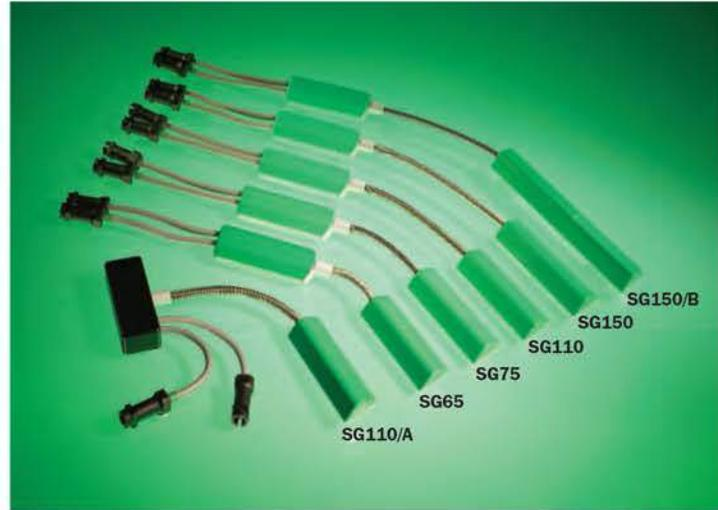
The comprehensive range of Biometrics' goniometers and torsionometers are ideal for quick, accurate measurements of joint movement in multiple planes. Extremely robust, lightweight and flexible, the sensors can be comfortably worn undetected under clothing, without hindering the actual joint movement of the subject.
