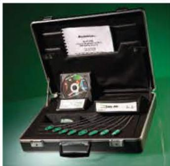
The Biometrics Ltd **Dynamometer** and **Pinchmeter** have been developed to provide precise scientific strength measurements in research and clinical settings. Applications include: bilateral strength testing for symmetry, pharmacological studies, work evaluations, clinical research, muscle strength/muscle fatigue monitoring, sustained grip and pinch testing.
