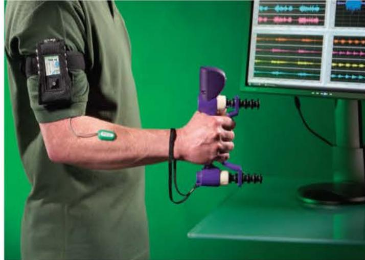
Strength measurements from the **P200 Pinchmeter** and **G200 Dynamometer** can readily be synchronized with data from other sensors such as EMG and goniometers connected to the **DataLOG**, **DataLINK**, and **K800**. Acquired data can be compared using the Biometrics Analysis Software or exported for analysis in other software.
