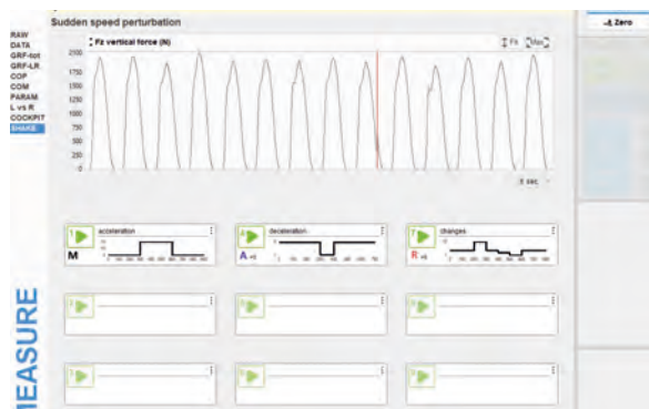
The perturbation mode called „shake“ will allow sudden speed changes to simulate slips and trips on the gaitway 3d.
