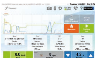
The MCU6 summary screen shows all relevant data of the workout including average and max. speed, elevation, duration and heart rate as well as biomechanical indicators as step lengths and cadence.
