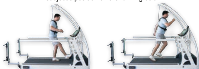
Sudden accelerations and stops of the running belt simulate slips (left) and trips (right)
