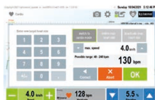
Cardio mode allows target heart rate in combination with maximum speed range definition for controlling the physical load by means of a combination of speed & elevation.
