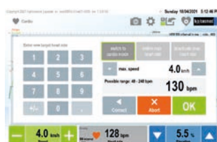
Cardio mode allows target heart rate in combination with maximum speed range definition for controlling the physical load by means of a combination of speed & elevation.
