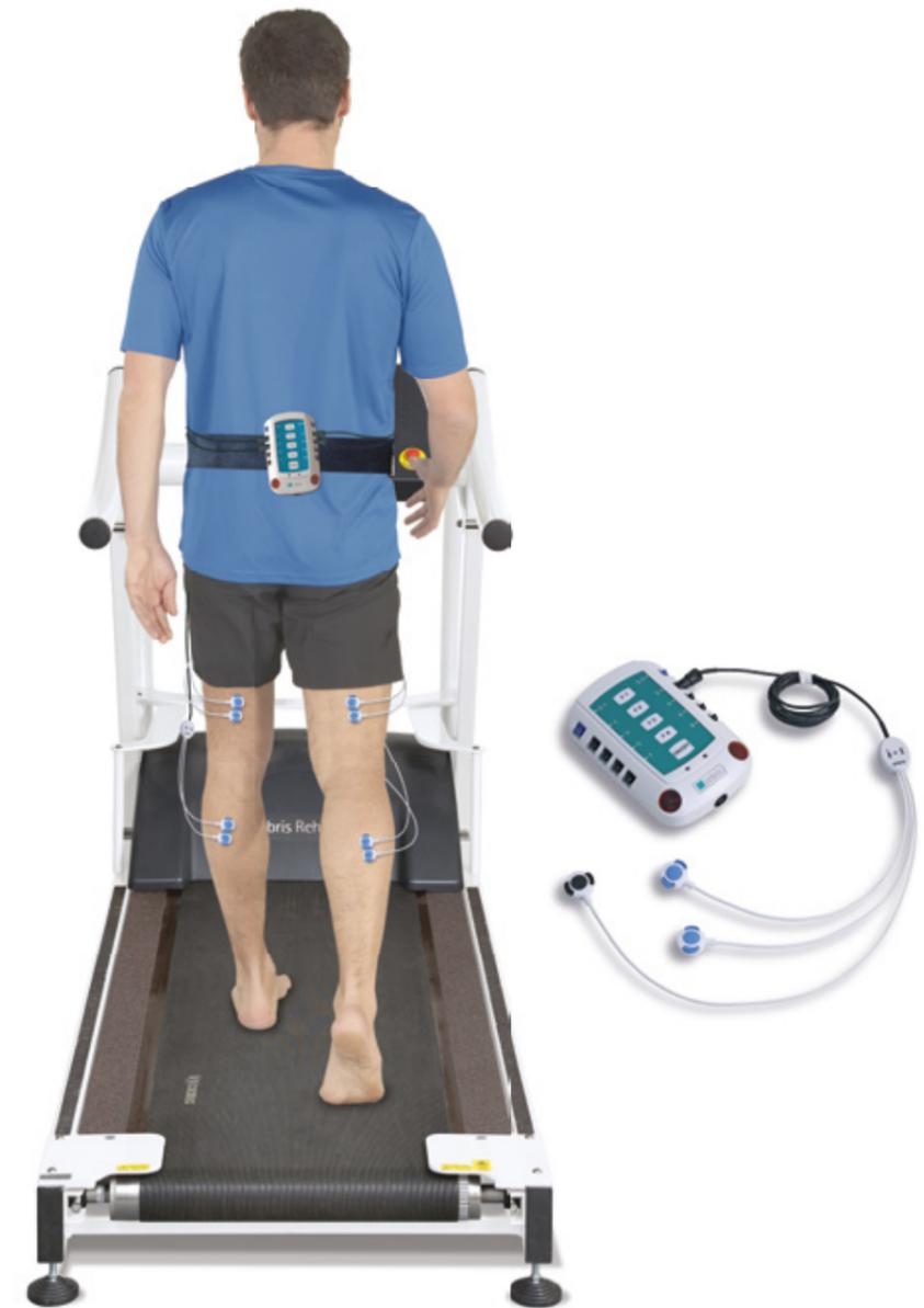
The fully synchronized zebris Myography system registers the muscle action potentials using bipolar electrodes placed on the skin surface. The Myography system comprises 8 measuring channels and is connected via Bluetooth to the evaluation computer. The evaluation report of the Rehawalk® system shows the time-standardized EMG signals.
