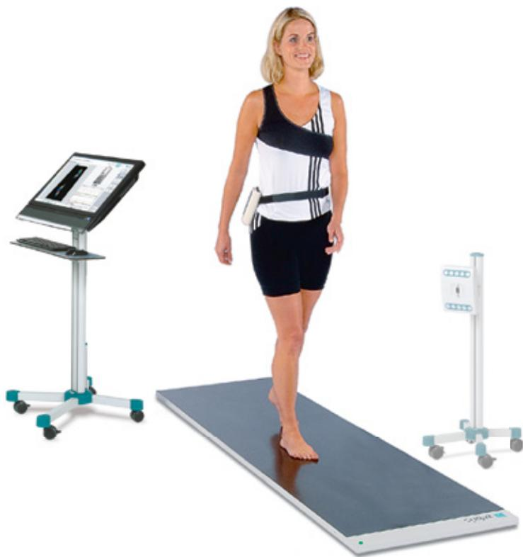
The zebris FDM measuring platforms for stance and gait analysis: 1.5 m - 6 m.
