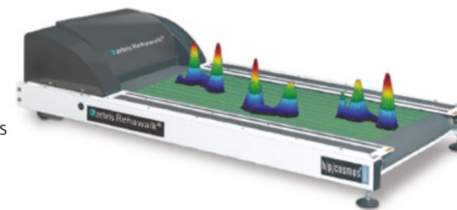
Underneath the belt, a pressure sensor matrix is installed featuring several thousand calibrated, capacitive pressure sensors. The belt movement is compensated for accurate measurement
